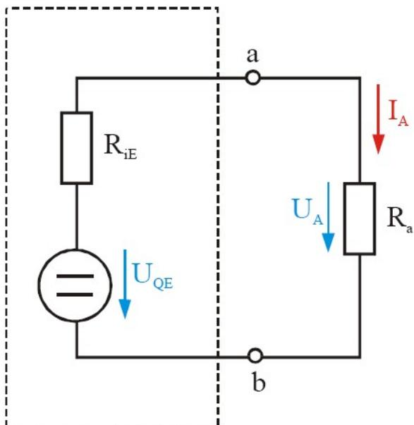
$$\underline{\underline{I_A}} = \frac{U_{QE}}{R_{iE} + R_a} = \frac{-7,5\text{V}}{300\Omega + 50\Omega} = \frac{-7,5\text{V}}{350\Omega} = \underline{\underline{-21,43\text{mA}}}$$
